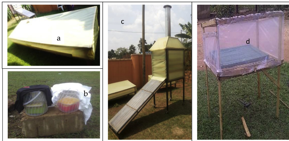
Figure 1. The four traditional solar drying methods and the proposed improved solar dryer. a) Convention Solar Drier (CSD) method, b) White-Cloth Shade (WCS) and Black-Cloth Shade (BCS) methods, c) Improved Solar Drier (ISD) method, and d) the traditional Open Sun Drying (OSD) method.
