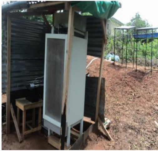
Figure 5: Solar photovoltaic powered evaporative cooling system (Olosunde et al. , 2016)
