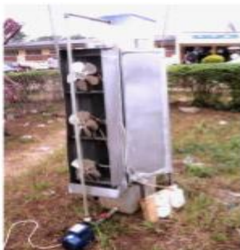
Figure 4: Schematic direct and active evaporative cooler (Chinenye, 2011; Chinenye et al. , 2013; Chinenye & Manuwa, 2014)
